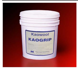
**Kaogrip** is a high temperature, air setting cement for use as an adhesive for ceramic fibre products. It sets to form a strong, hard film that develops a ceramic bond at high temperatures, yet maintains excellent resistance to thermal shock.
